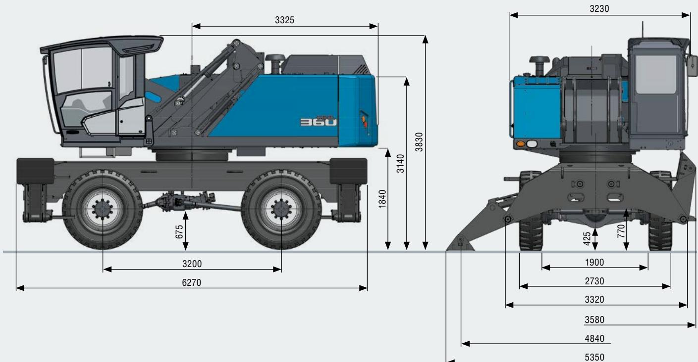
**DIMENSIONS | ABMESSUNGEN | DIMENSIONS | DIMENSIONES | DIMENSIONI | DIMENSÕES [mm]**
