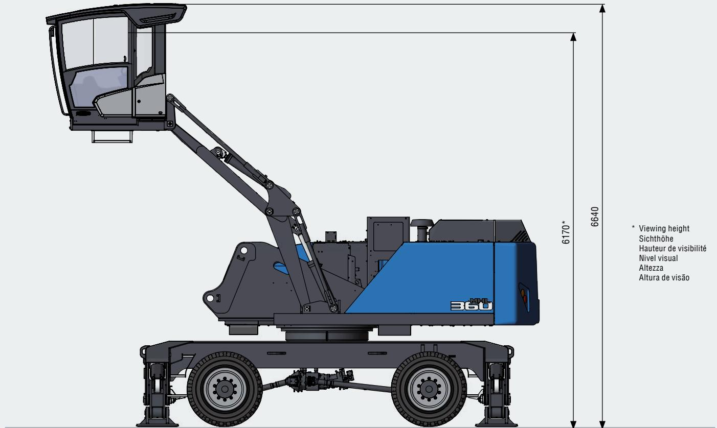
**TRANSPORT DIMENSIONS | TRANSPORTABMESSUNGEN | DIMENSIONS DE TRANSPORT [mm]****DIMENSIONES DE TRANSPORTES | DIMENSIONI DI TRASPORTO | DIMENSÕES DE TRANSPORTE [mm]**
