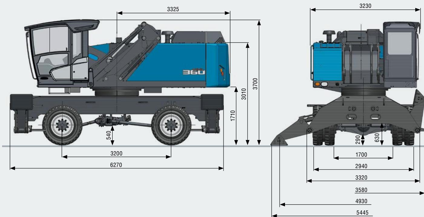
**TRANSPORT DIMENSIONS | TRANSPORTABMESSUNGEN | DIMENSIONS DE TRANSPORT [mm]**
