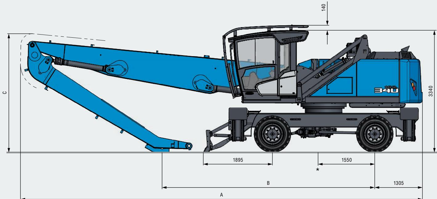
Transport position with dozer blade; undercarriage rotated by 180°
